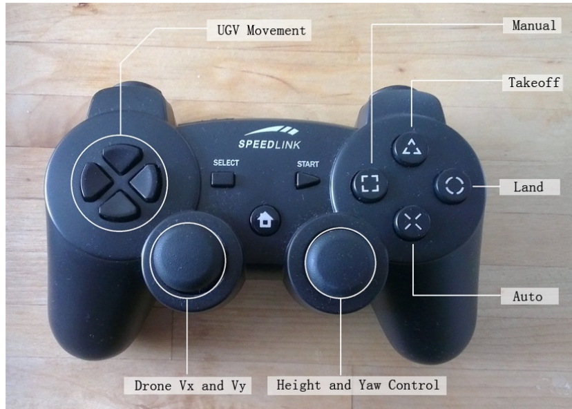
Fig. 6.3: The joystick used for teleoperating the UAV. The operator can control 4 DOF of the AR. Drone and send taking off / landing command to the drone. It is also able to switch between autonomous and manual flight mode by pressing the corresponding buttons.
