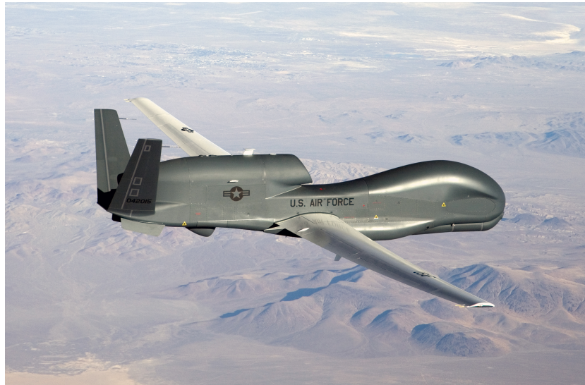
Fig. 1.1: Global Hawk 1 by U.S. Air Force photo by Bobbi Zapka. Global Hawk is one of the most famous military UAV platform. It has a cruising altitude of 60,000 ft and a maximum speed of approximately 575 km/h. Picture reproduced from [40].
