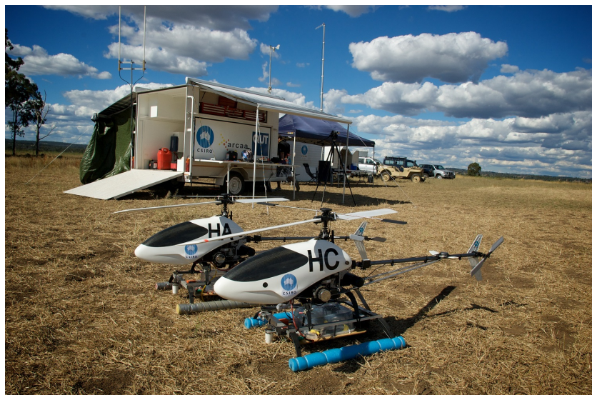
Fig. 1.2: ResQu Unmanned Aircraft designed to help fighting natural disasters in Australia. Reprinted from http://www.unmannedsystemstechnology.com/ .
