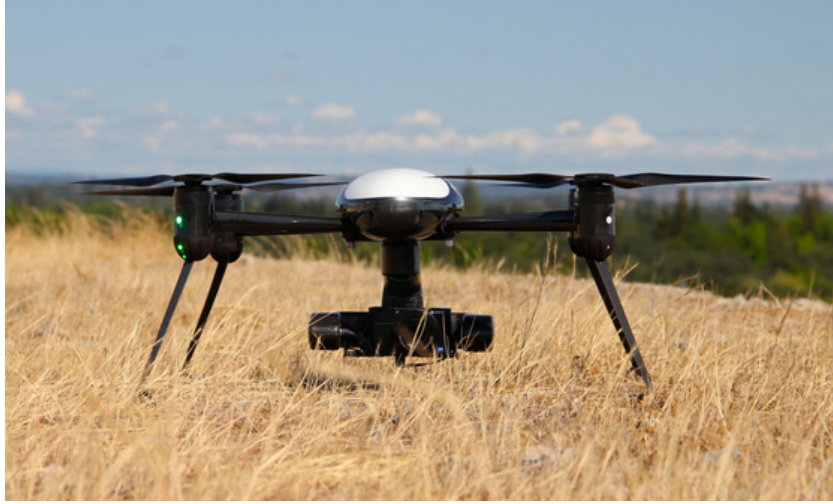
Fig. 1.6: The DragonFly X4-ES Quadcopter. This quadcopter is specifically designed for public safety use and has a vibration isolated camera gimble which permits to delivery high-quality real-time video[9].
