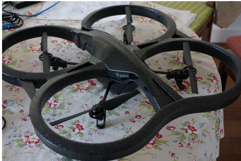
Fig. 3.3: The AR.Drone 2.0 quadcopter developed by Parrot SA, France
